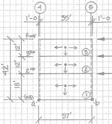
MAJORITY OF LOAD DISTRIBUTED TO THIS WALL. SEE SEISMIC LOAD DISTRIBUTION SUMMARY AT THE BEGINNING OF THIS SECTION.
