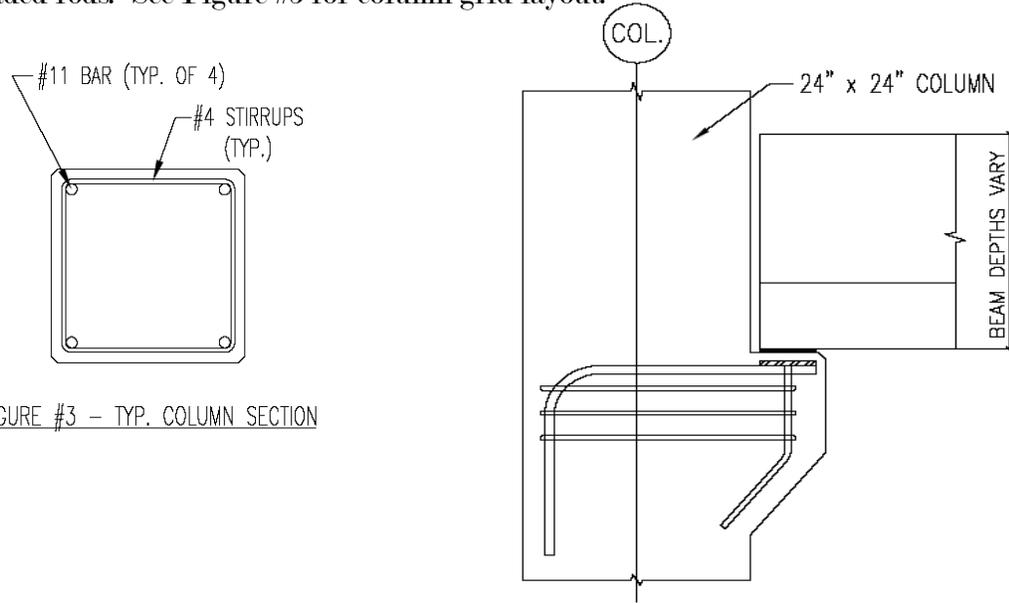
FIGURE #3 - TYP. COLUMN SECTION
