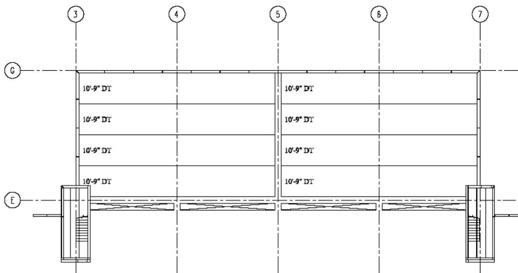
FIGURE #6 - LOW ROOF DT LAYOUT
